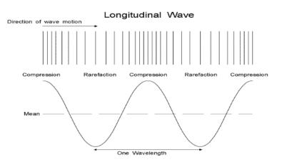
The above diagram shows a sound wave traveling from left to right. The vertical bars represent thin slices of the medium which are displaced to form areas of compression and rarefaction. The sine wave represents their displacement relative to their mean position. The distance over which the vibration repeats itself is called the wavelength. The number of complete vibrations in one second is called the frequency of the sound wave. The velocity of sound in the medium is given by:
